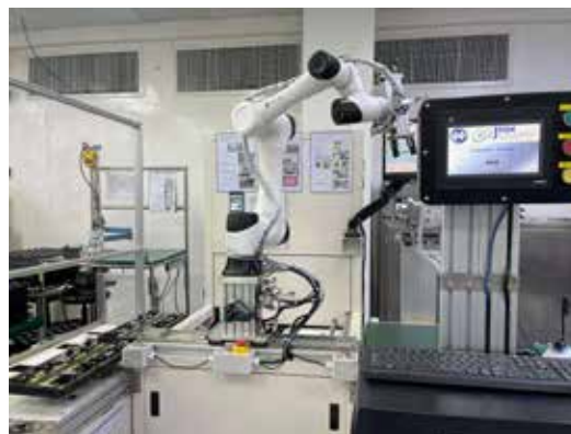
In-house robotic optical and electrical tester
